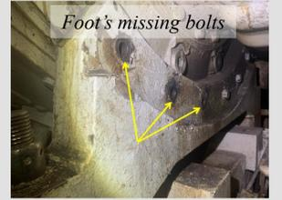
These faults are thought to be caused by the high vibrations of the turbocharger
